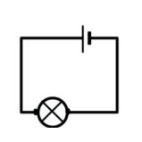
Circuit: An electrical circuit is a path or line through which an electrical current flows
