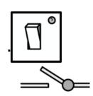
Switch: an electrical component that can "make" or "break" an electrical circuit
