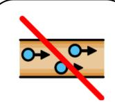
Insulator (electrical): an insulator is a material whose internal electric charges do not flow freely.
