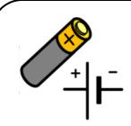
Battery: a device that stores chemical energy and makes it available in an electrical form
