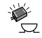
Buzzer: an automatic signalling device. They are used as alarms and door bells.
